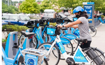
At a docking station, users can distinguish e-bikes from conventional bicycles by the frame color; the former are white and the latter are blue. Image courtesy of Indego.
